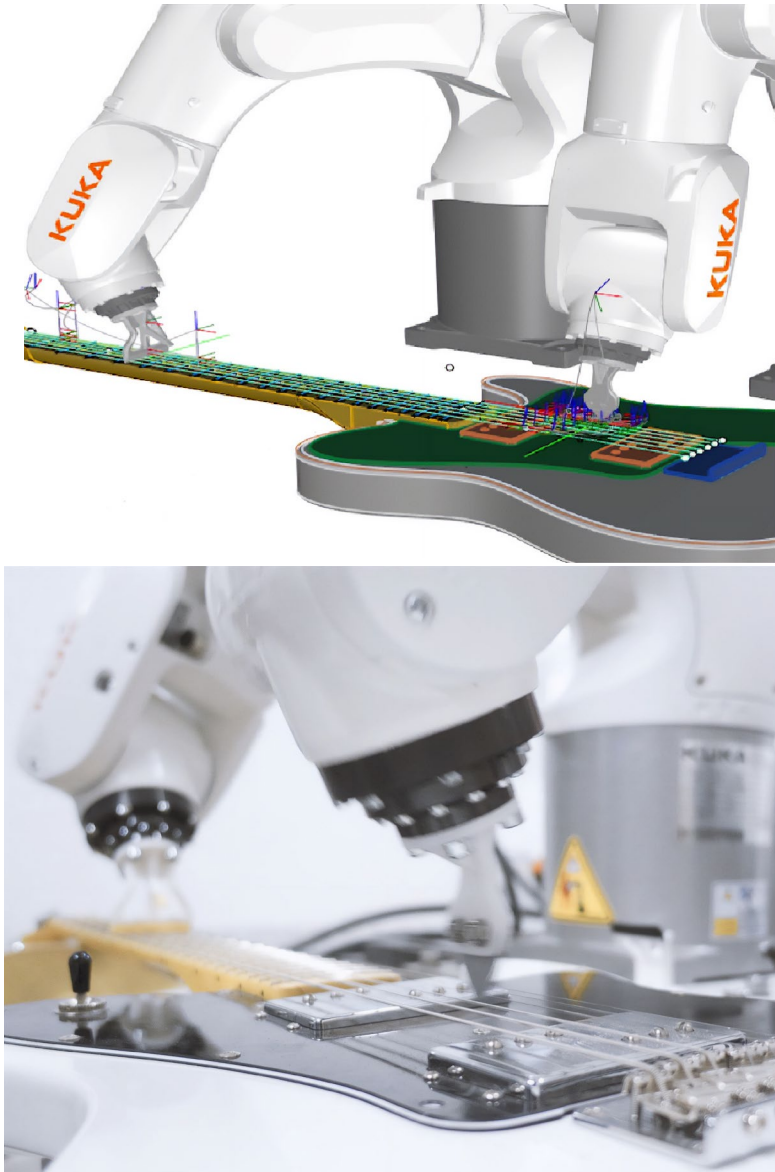
Figure 54: Guitar playing simulation (top) and prototypes with 3D-printed endeffectors (bottom).
