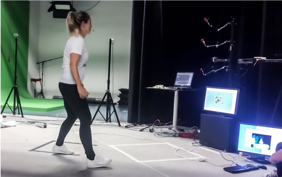
Figure 38: Live robot pre-visualization during motion capture through KUKA|prc and a Kinect-2 sensor.
