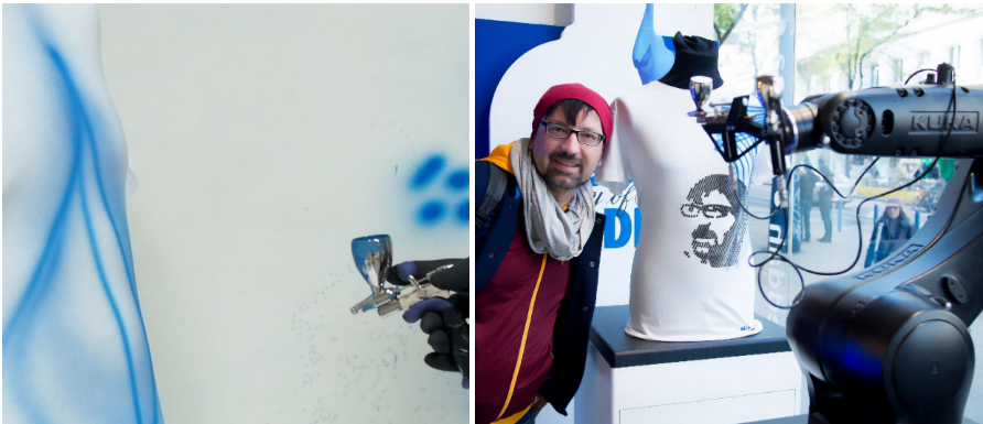
Figure 45: Manual prototype (left), robotically fabricated result with static air pressure, varying only distance and speed (right).
