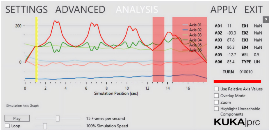
Figure 24: Visualization of toolpath analysis for excessive speed/singularities (yellow) and unreachable positions (red).
