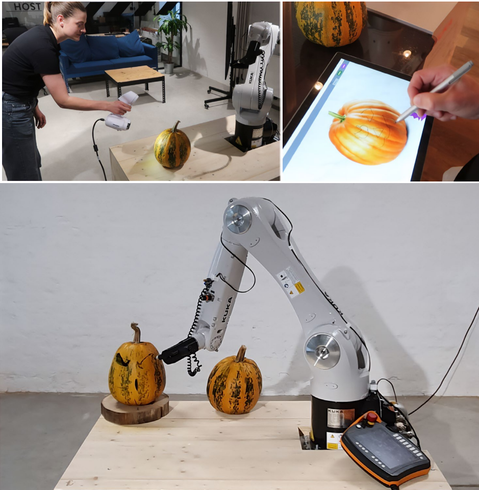
Figure 57: Workflow to apply a 2D pattern onto a free-formed surface.
