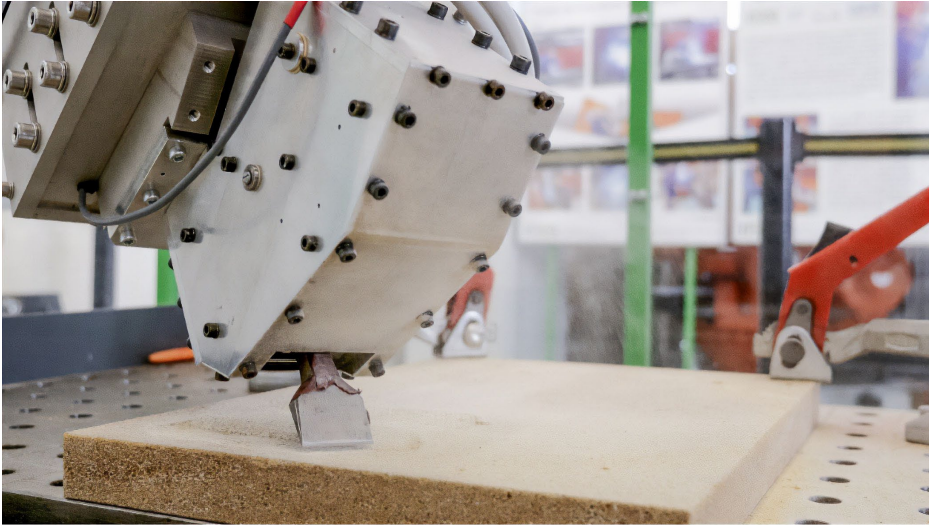
Figure 42: Stone chiseling process developed through the AROSU project.
