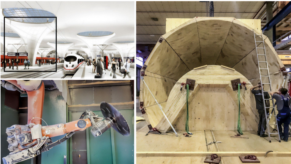
Figure 53: Parametric robot control at Züblin Timber (Züblin Timber).
