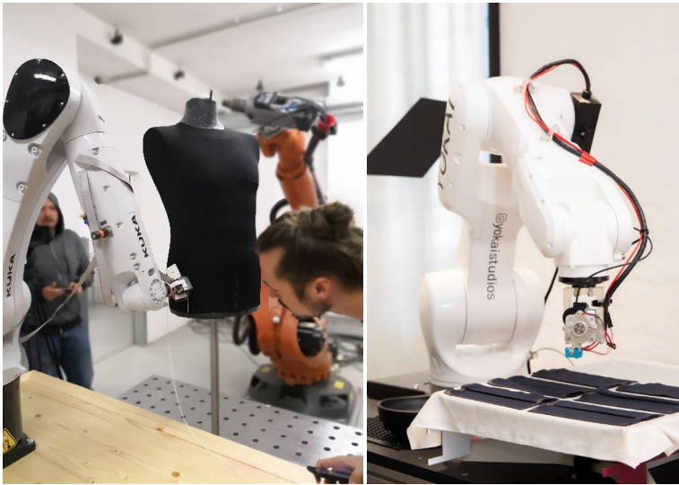
Figure 52: Connection and decoration of textiles via additive manufacturing technologies. From prototype (left) to automated production of face masks during the COVID-19 pandemic (right, Yokai Studios).
