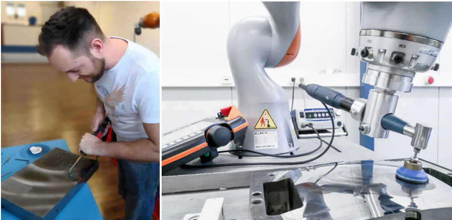
Figure 47: Manual polishing (left), developed robotic process (right).
