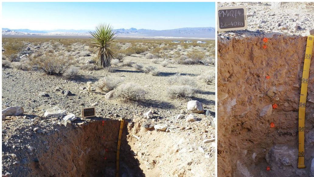
FIGURE 9 Soil profile in a Late Pleistocene alluvial fan in the Providence Mountains piedmont, Mojave Desert, belonging to a soil chronosequence investigated by McDonald et al. (1996) and McDonald, McFadden, and Wells (2003). The profile has the horizon sequence Vk-Btk-Bk-Ck-C, whereby the clay in the Btk horizon and most of the pedogenic carbonate below 75 cm depth accumulated under the moister conditions of the Late Pleistocene (McDonald et al., 1996; McDonald, McFadden, & Wells, 2003).
