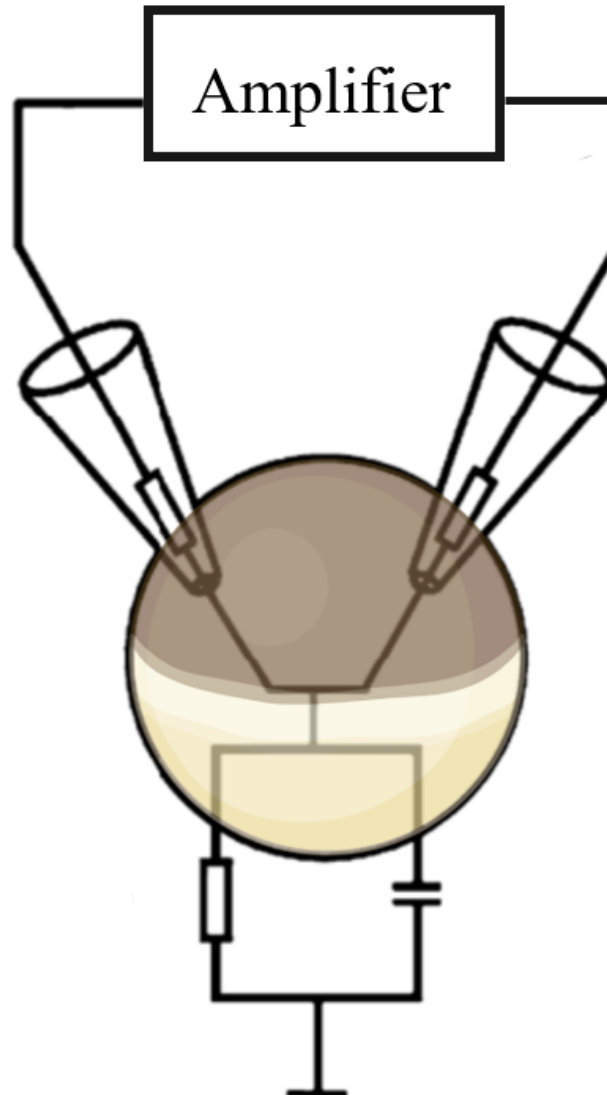
Figure 3.3: Schematic demonstration of the TEVC employed on a Xenopus oocytes.
