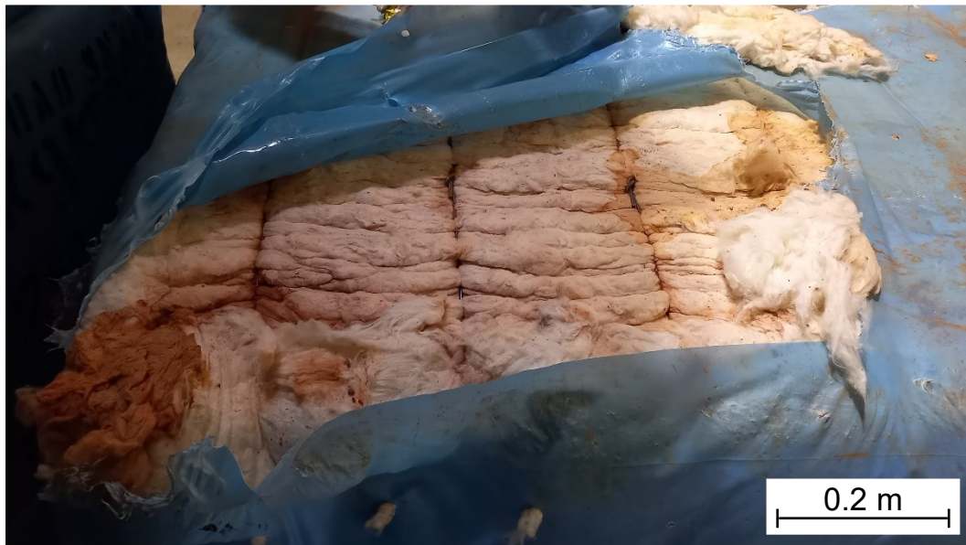
Fig. 5.6: Contaminated cotton by dust and rust [KFS22]
