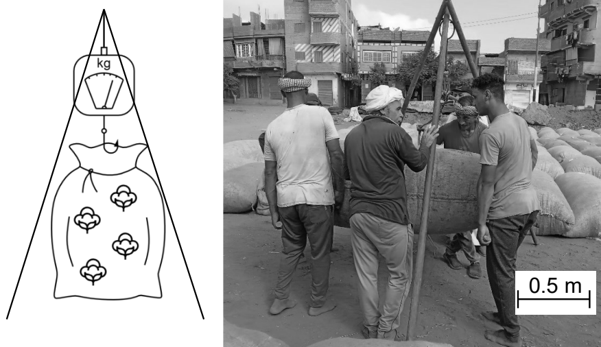
Fig. 5.2: 280 kg raw seed cotton bag handling with four persons and tools
