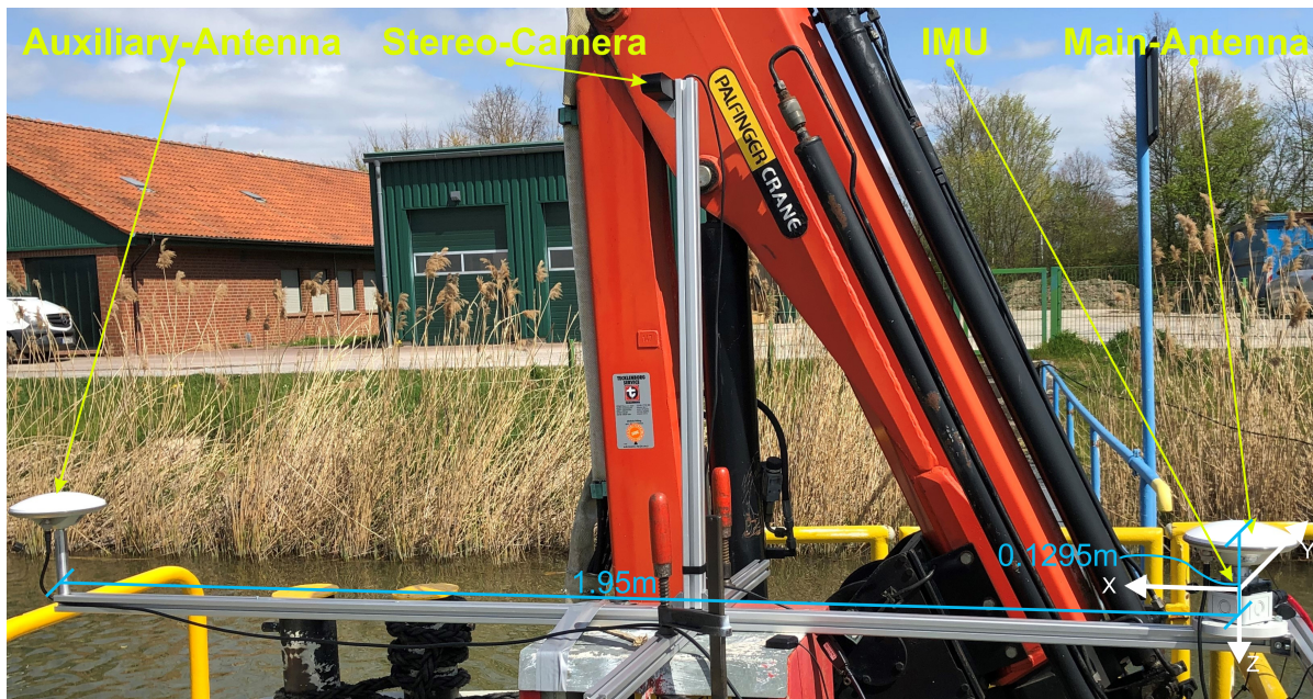
(a) Test Vehicle 1: Measurement setup on the ship "Datteln" with the primary antenna mounted on the top of IMU box
