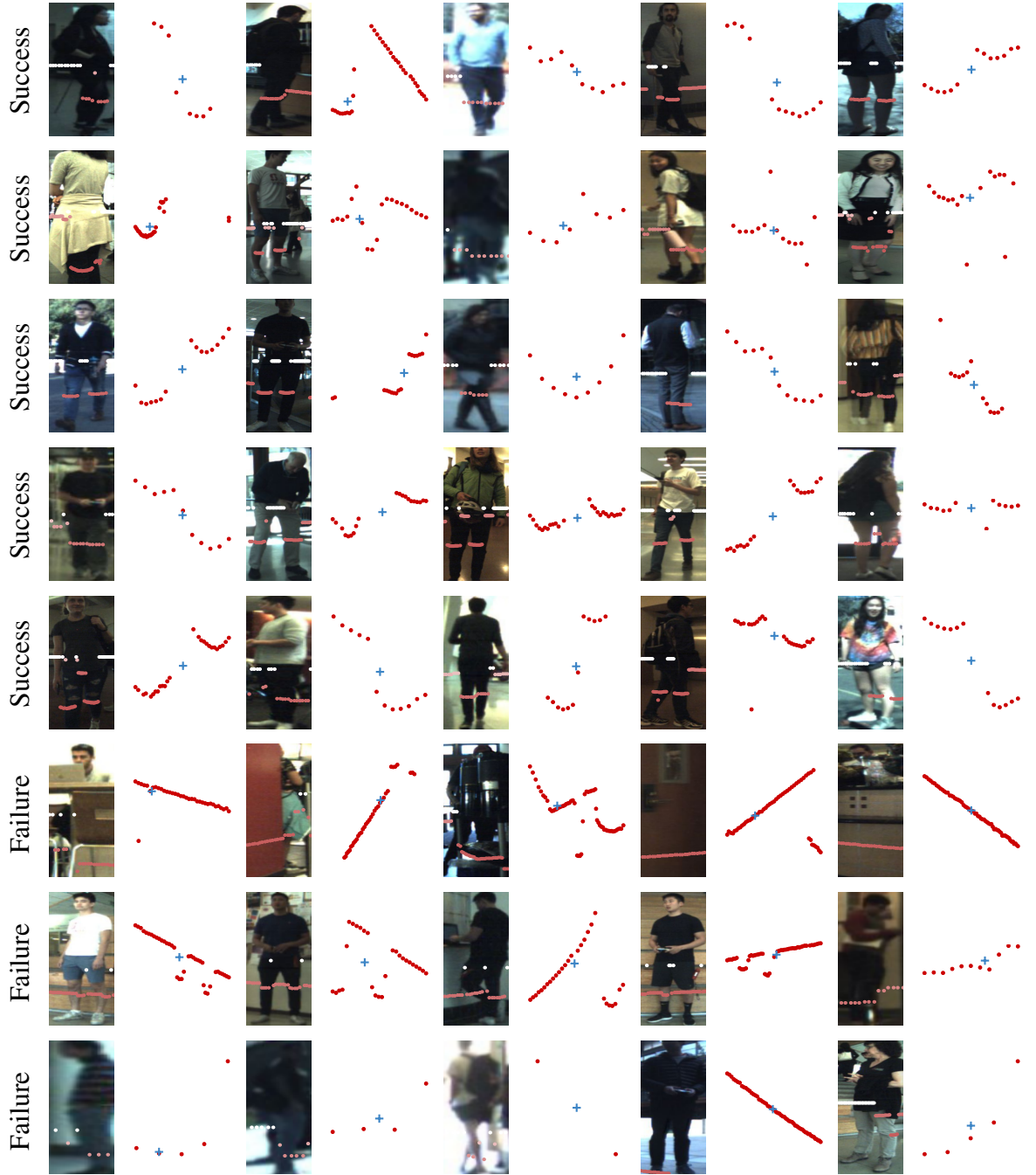
Figure 5.2: Person detections and the top-down view of the matching pseudo-labels (+) with surrounding LiDAR points (within a 0.5\text{ m} radius). The LiDAR points are overlaid in the detection images, where the color encodes measured distance with red being closest and white being farthest. Common failure cases are shown in the bottom three rows: heavy occlusion (row 6); background distraction (row 7); sparse LiDAR points at far distance (row 8, column 1-3); and faulty calibration or synchronization between sensors (row 8, column 4-5).
