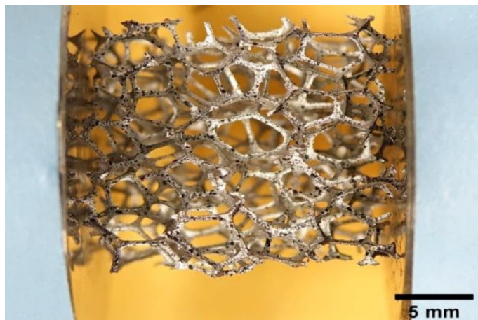
Figure 4-5- A sprinkled foam specimen fixed between the compression plates.
