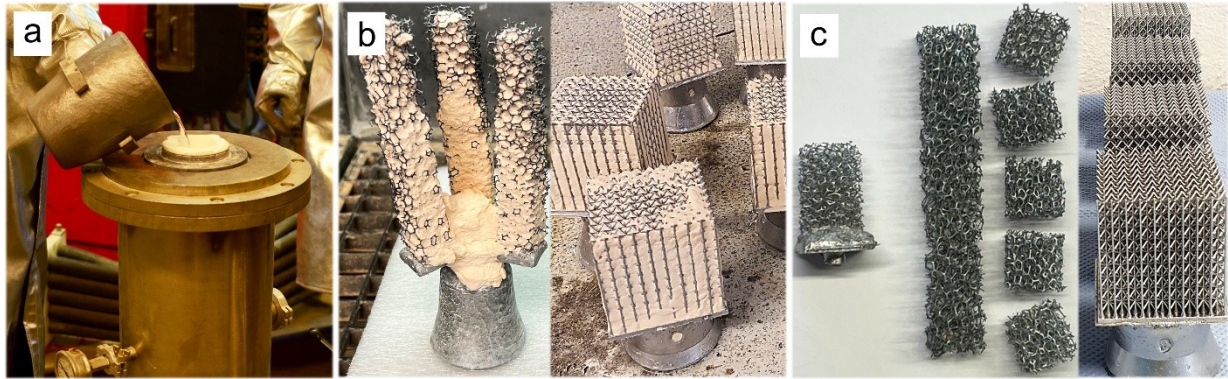
Figure 4-4- a) Casting with the help of under pressure, b) casting products after demolding using water stream, and c) final cast specimens after complete removal of the molding material.
