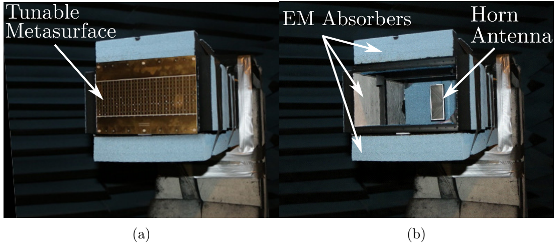
Fig. 4.24: Measurement setup of the fabricated metasurface together with the horn antenna. (a) Tunable metasurface illuminated by the horn. (b) Horizontally polarized horn antenna without the tunable metasurface.
