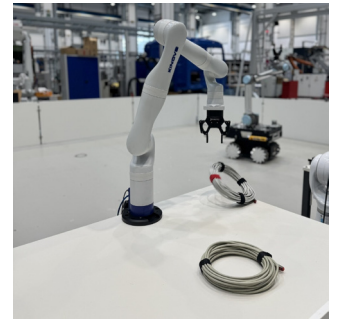
(f) Robot arm placing the cable.
