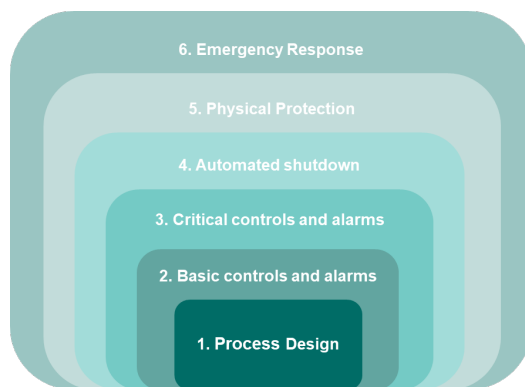
Figure 11: Overview of the different levels within the Layers of Protection Analysis (LOPA) as adapted from R. J. Willey. [203]
