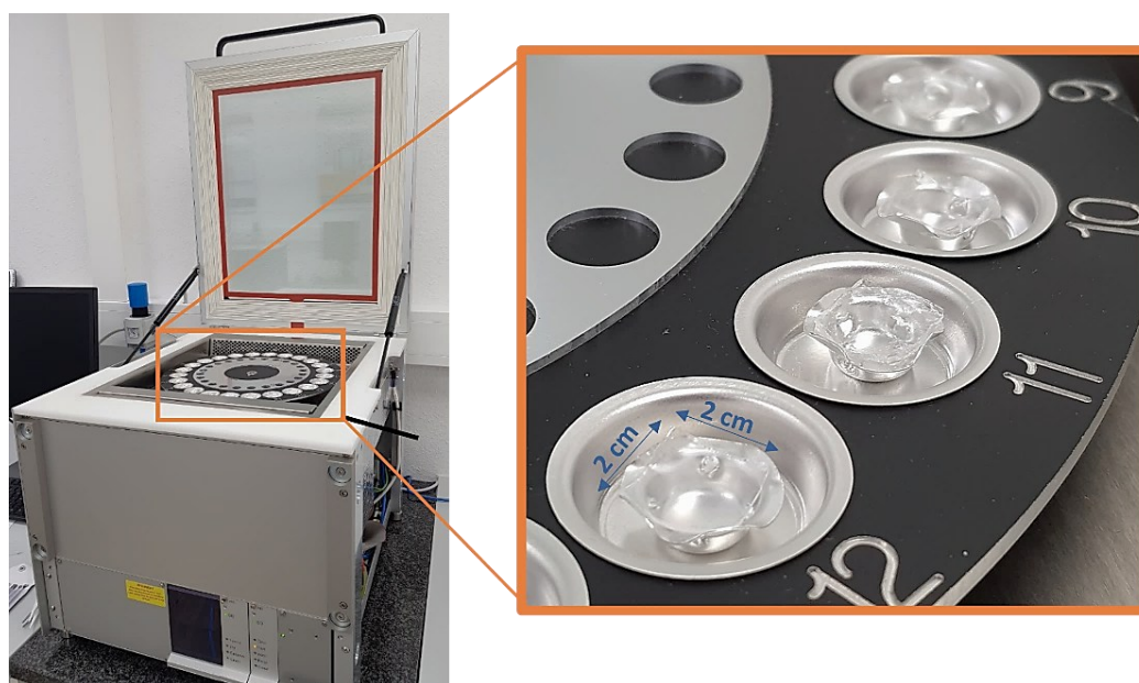
Figure 5-2: Setup of the SPSx-1 \mu -Advance water vapor sorption system from ProUmid GmbH & Co. KG, featuring a sample tray with 23 positions in a climate chamber with an integrated microbalance.
