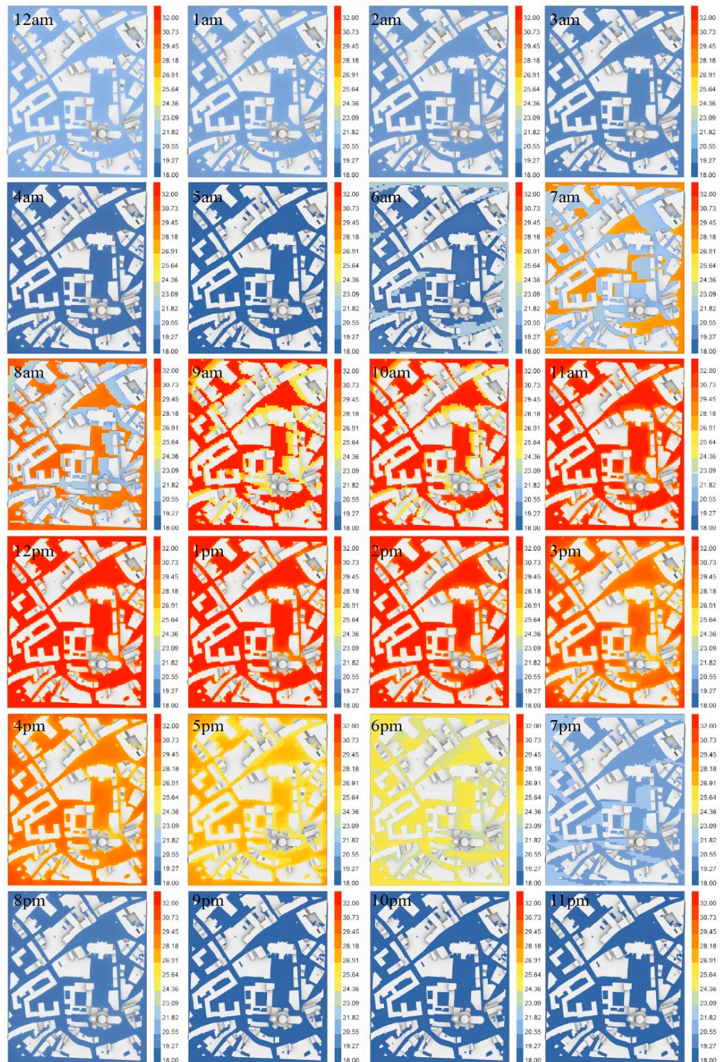
Figure A2. Hourly UTCI maps for Typo-Morphology 1 (compact morphology) under the RCP 8.5 climate scenario in 2050.
