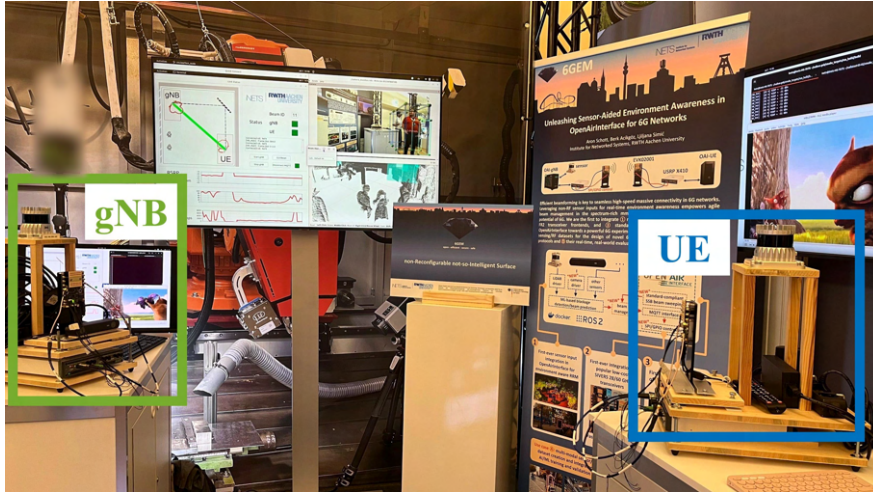
Figure 3.1: The testbed for (1) being demonstrated at the Berlin 6G Conference 2025, with the gNB and UE indicated.
