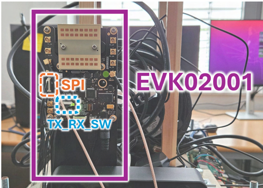
Figure 3.4: The EVK02001 with important components illustrated.
