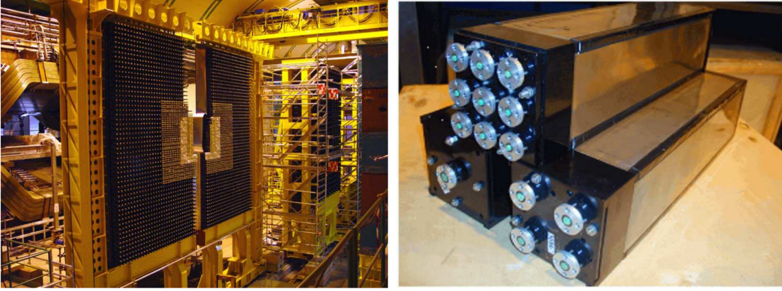
Figure 4.9: Picture of the ECAL in the detector cavern (left) and ECAL modules from different detector regions (right). The figures are taken from Ref. [16].
