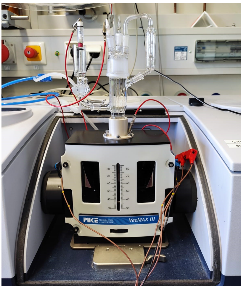
Figure 4.10: Picture of the H-cell in the ATR setup.
