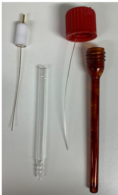
Figure 4.1: Reference electrode compartments used in this work. The commercially available one used for the comparison of Ag-based REs (left) and the darkened glass vial to inhibit the \text{Ag}^+ precipitation for the ion influence study (right). Picture taken from the Bachelor thesis of Anne Liang. [160]
