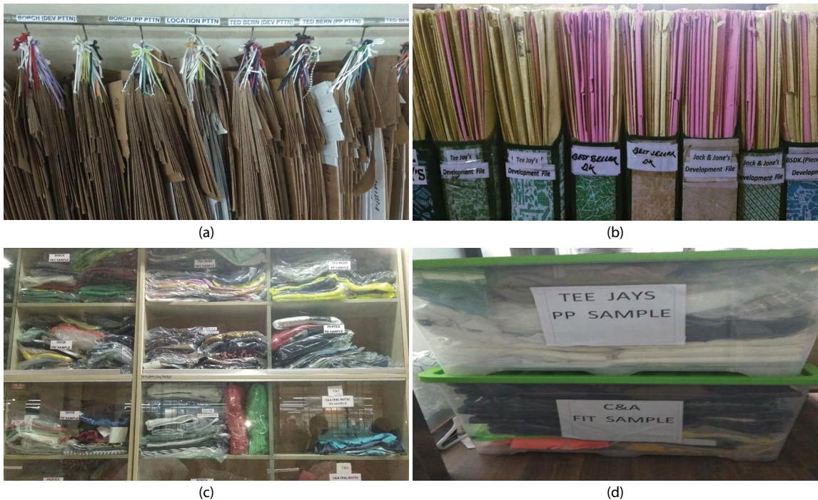
Figure 6: Newly ordered sewing floor of product development section: a) labelling of cut patterns, b) labelling of files, c) labelling of counter samples storage, d) plastic bin with labelling of past style items
