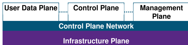
FIGURE 13. High-level architecture: The user, control and management planes run on the network infrastructure, connected in a control plane network for management and control communication.
