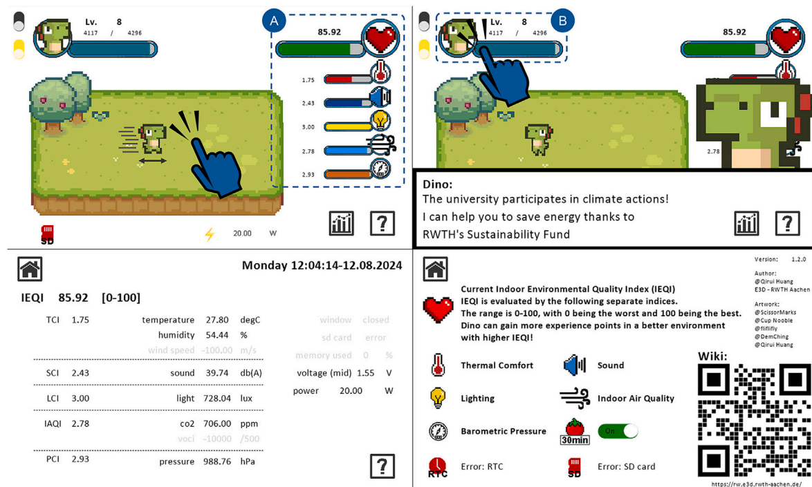
Fig. 5. Overview of the GUI. Top left: main screen with gamification elements; Top right: example of the feedback system; Bottom left: sensor data page (unconfigured sensors are displayed in gray); Bottom right: help page with a brief description and a QR code linking to the wiki page. Area A displays all comfort indices, and area B shows the current level and XP. In addition to automatic feedback provided every 30 minutes, users may tap area B to request feedback manually. (For interpretation of the references to colour in this Figure legend, the reader is referred to the web version of this article.)
