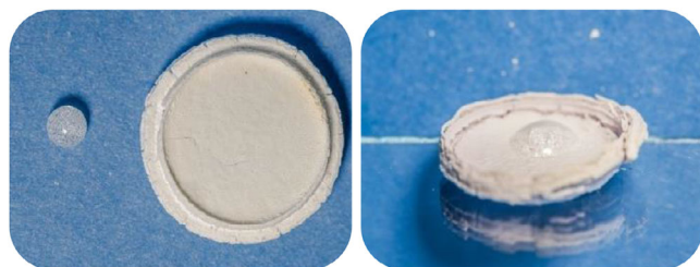
FIGURE 3 | Photographs of substrate and glass after the heating microscopic trial for tantalum (left) and niobium (right).
