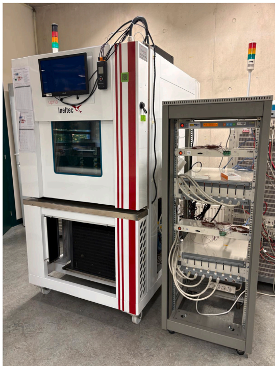
Fig. 2. Experimental setup, consisting of a battery tester and a thermal chamber, in the Laboratory for Energy Storage and Microgrids of the Public University of Navarre (UPNA).
