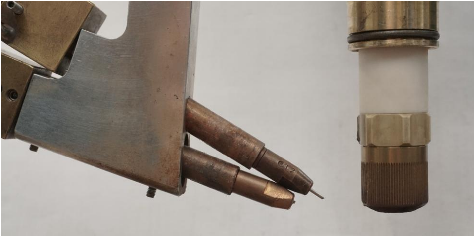
Figure 2: Multi-material welding torch with a fixture for two wires on the left and a plasma torch on the right
