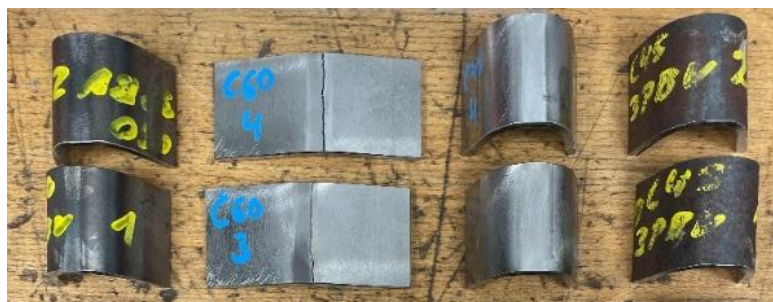
Figure 10: Left side: C60, right side: C45. Fracture pattern of the top-side specimens with martensitic brittle fracture pattern of C60. C45 shows no fracture pattern.
