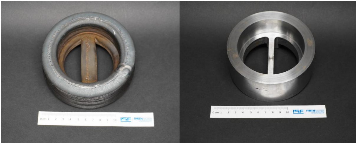
Figure 5: Demonstrators: low-alloy steel on the left, multi-material strategy on the right
