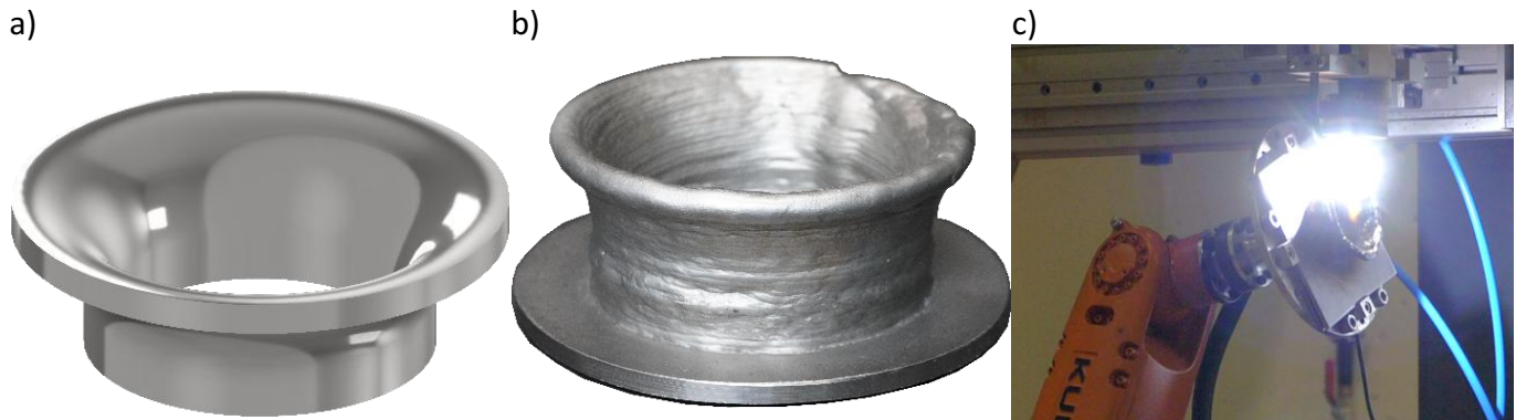
Figure 8: a) CAD model of the nozzle, b) manufactured nozzle, c) manufacturing process of the 34th layer
