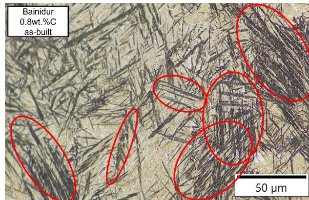
Figure 5: Bainidur 0.8 wt.% C as-built microstructure with lath bundles.
