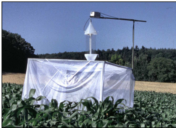
Figure 7. Light trap linked to a cage.
