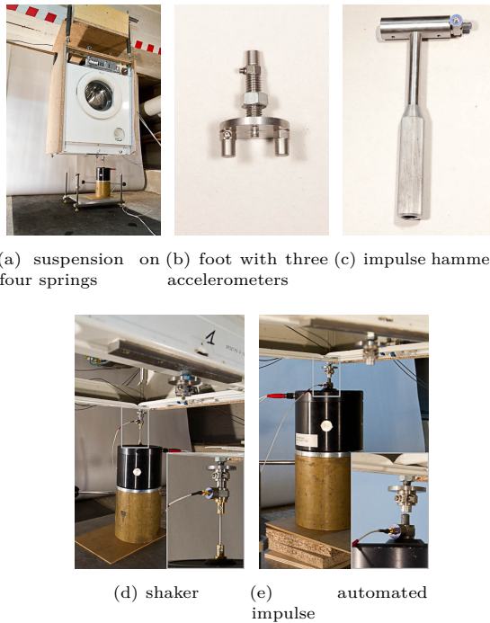
Figure 5.9: Setup of three different excitation sources for the source mobility measurements.
