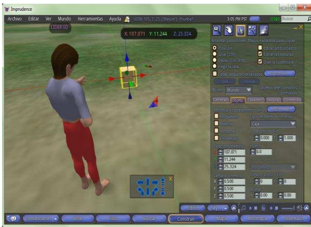
Fig. 7. OpenSim viewer, basic tools menus and tabs for designing objects in the virtual worlds.
