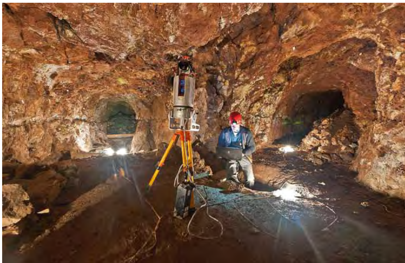
The documentations inside the complex mine are time-consuming. Here a 3D scanner by Arcton is used (photo: K. Stange/AVttention).
