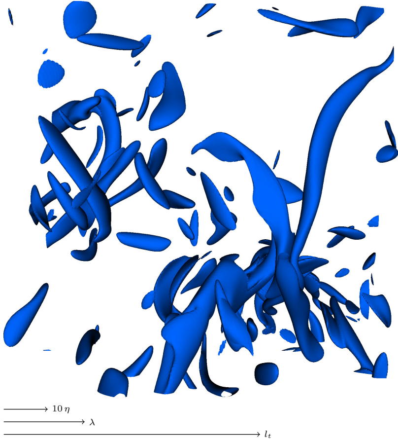
Figure 3.6: Three-dimensional iso-surface (top-view) of the normalized enstrophy \omega^2/\langle\omega^2\rangle , where the value of the iso-surface equals 8, for case R1. A magnification of the bottom left corner of size \pi/2 \times \pi/2 \times \pi/2 or 256 \times 256 \times 256 grid points, respectively, is shown.
