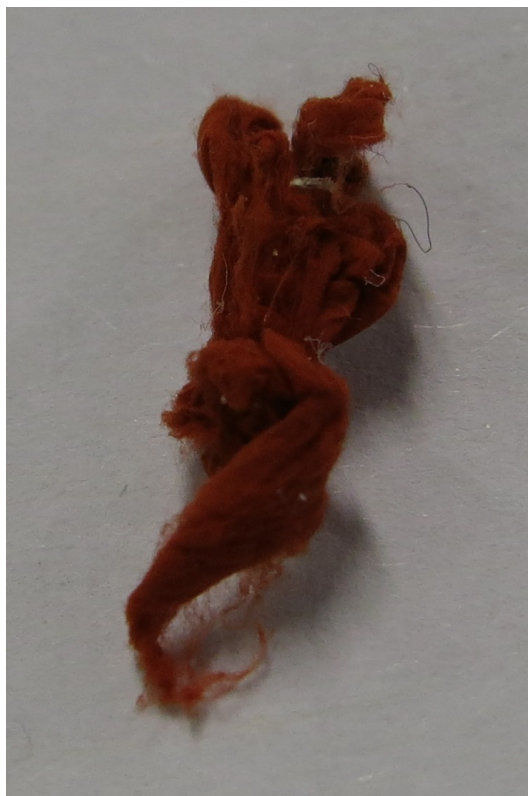
Figure 75: Photo of PCL-microfibres with iron(III) oxide nanoparticles; the red colour of the fibres due to the pigmentation with the nanoparticles is clearly visible
