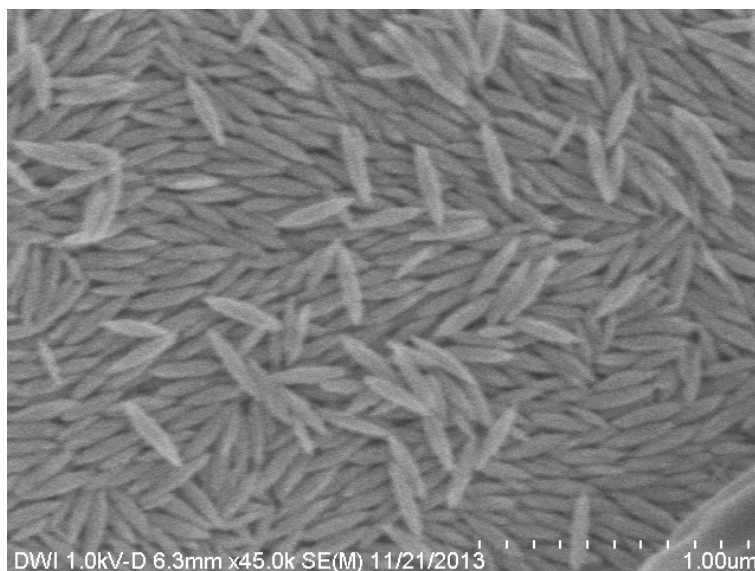
Figure 72: FESEM micrograph of iron(III) oxide nanoparticles
