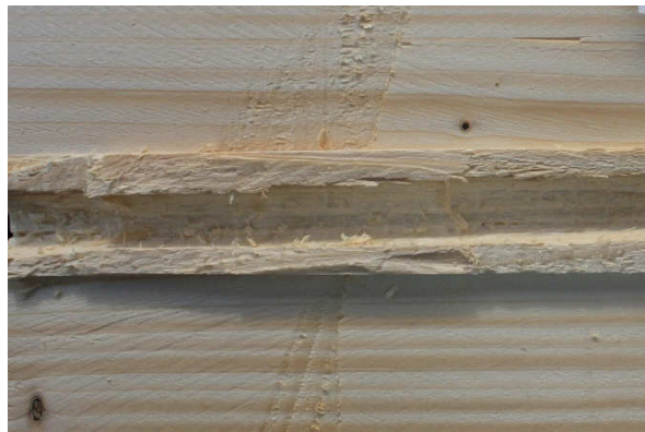
f) Probe P-24-12-0-3 d_s = 12 \text{ mm} , \alpha = 0^\circ , l_p = 240 \text{ mm}
