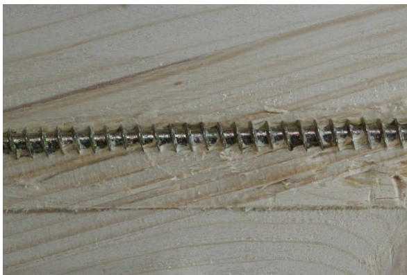
e) Probe P-16-8-15-1 d_s = 8 \text{ mm} , \alpha = 15^\circ , l_p = 160 \text{ mm}
