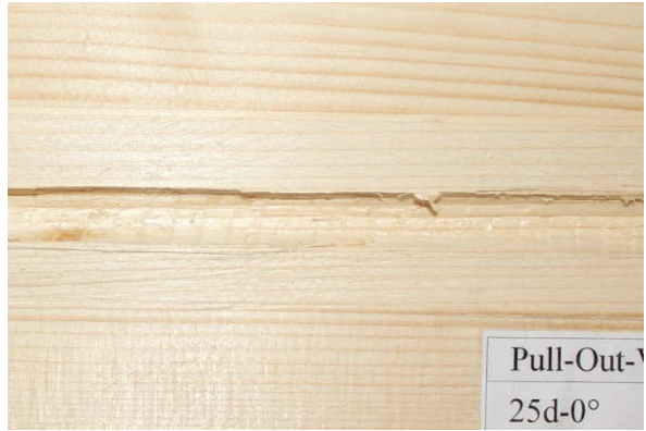
b) Probe P-30-12-0-1 d_s = 12 \text{ mm} , \alpha = 0^\circ , l_p = 300 \text{ mm}
