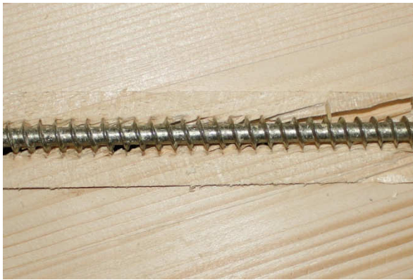
a) Probe P-20-10-15-2 d_s = 10 \text{ mm} , \alpha = 15^\circ , l_p = 200 \text{ mm}
