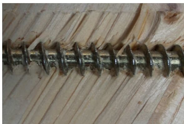
d) Probe P-24-12-6-3 d_s = 12 \text{ mm} , \alpha = 60^\circ , l_p = 240 \text{ mm}
