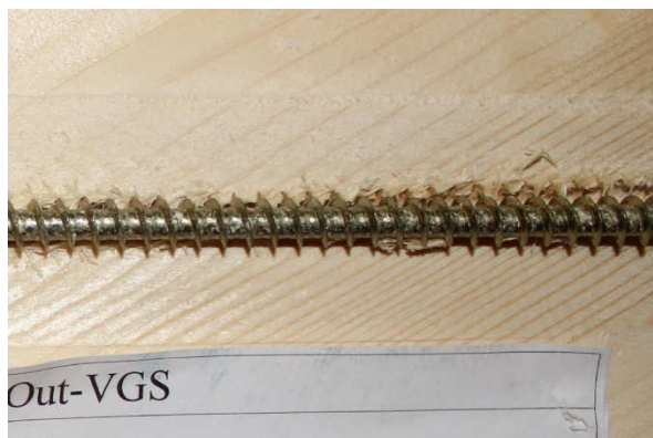
f) Probe P-20-8-3-1 d_s = 8 \text{ mm} , \alpha = 30^\circ , l_p = 200 \text{ mm}
