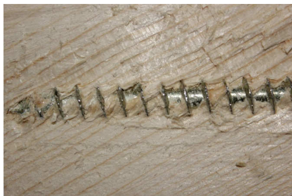
f) Probe P-S-20-10-3-1 d_s = 10 \text{ mm} , \alpha = 30^\circ , l_p = 200 \text{ mm}
