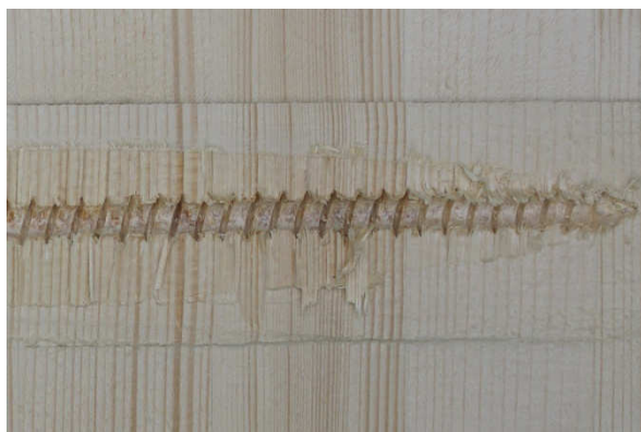
c) Probe P-20-10-9-1 d_s = 10 \text{ mm} , \alpha = 90^\circ , l_p = 200 \text{ mm}
