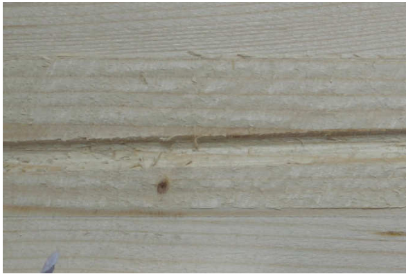
a) Probe P-12-8-0-1 d_s = 8 \text{ mm} , \alpha = 0^\circ , l_p = 120 \text{ mm}
