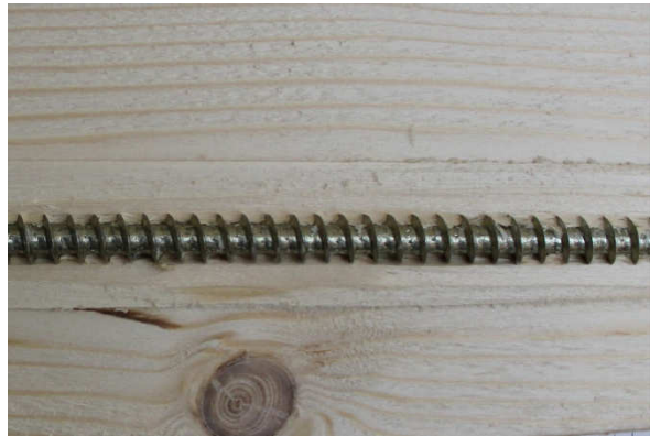
d) Probe P-20-8-0-3 d_s = 8 \text{ mm} , \alpha = 0^\circ , l_p = 200 \text{ mm}
