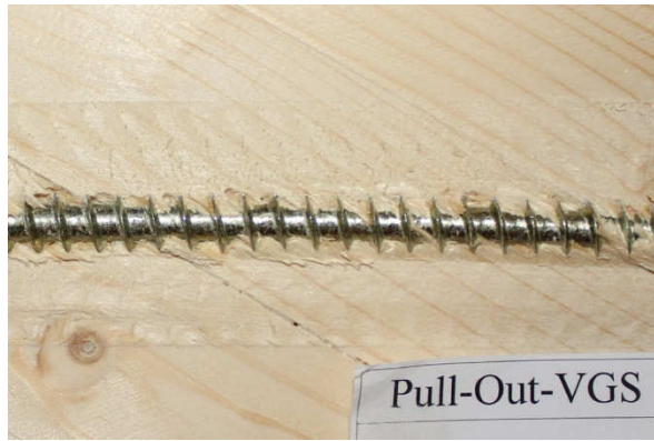
b) Probe P-25-10-3-1 d_s = 10 \text{ mm} , \alpha = 30^\circ , l_p = 250 \text{ mm}
