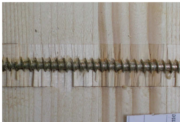
d) Probe P-16-8-9-3 d_s = 8 \text{ mm} , \alpha = 90^\circ , l_p = 160 \text{ mm}
