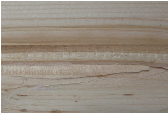
c) Probe P-15-10-0-2 d_s = 10 \text{ mm} , \alpha = 0^\circ , l_p = 150 \text{ mm}
