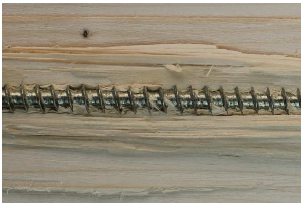
e) Probe P-20-10-0-2 d_s = 10 \text{ mm} , \alpha = 0^\circ , l_p = 200 \text{ mm}
