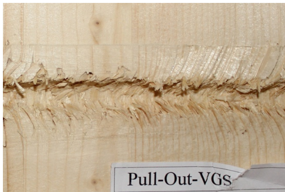
a) Probe P-18-12-9-1 d_s = 12 \text{ mm} , \alpha = 90^\circ , l_p = 180 \text{ mm}
