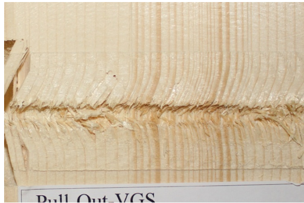
b) Probe P-12-8-9-1 d_s = 8 \text{ mm} , \alpha = 90^\circ , l_p = 120 \text{ mm}
