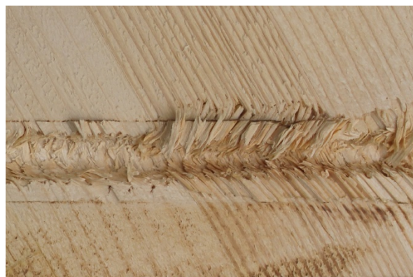
f) Probe P-15-10-6-2 d_s = 10 \text{ mm} , \alpha = 60^\circ , l_p = 150 \text{ mm}
