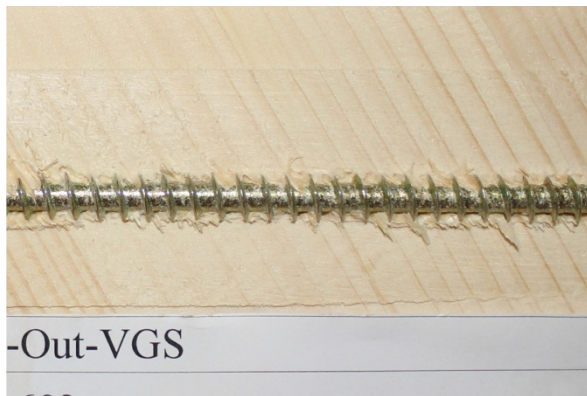
a) Probe P-16-8-6-2 d_s = 8 \text{ mm} , \alpha = 60^\circ , l_p = 160 \text{ mm}
