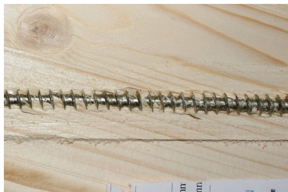
f) Probe P-20-8-15-1 d_s = 8 \text{ mm} , \alpha = 15^\circ , l_p = 200 \text{ mm}
