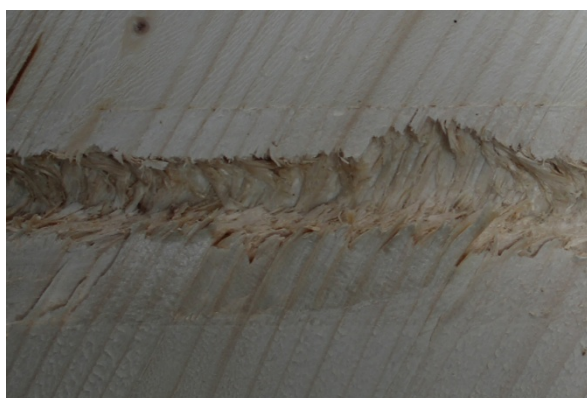
e) Probe P-24-12-6-2 d_s = 12 \text{ mm} , \alpha = 60^\circ , l_p = 240 \text{ mm}
