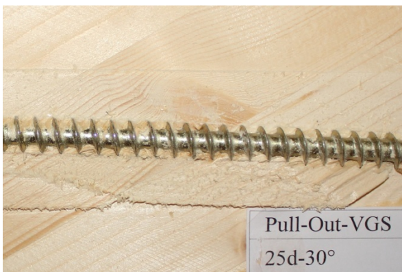
c) Probe P-30-12-3-3 d_s = 12 \text{ mm} , \alpha = 30^\circ , l_p = 300 \text{ mm}
