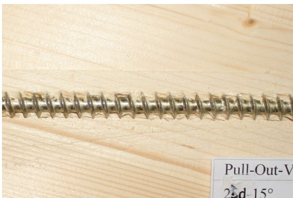
c) Probe P-30-12-15-2 d_s = 12 \text{ mm} , \alpha = 15^\circ , l_p = 300 \text{ mm}
