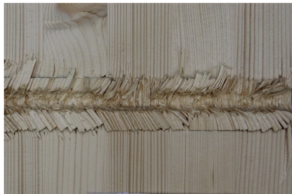
b) Probe P-R-18-12-9-3 d_s = 12 \text{ mm} , \alpha = 90^\circ , l_p = 180 \text{ mm}
