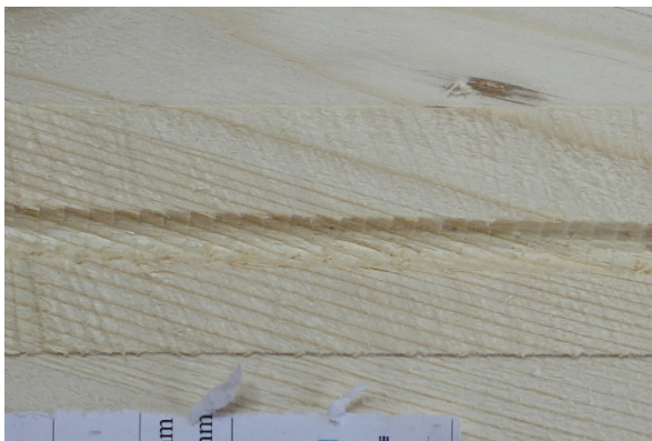
c) Probe P-12-8-15-1 d_s = 8 \text{ mm} , \alpha = 15^\circ , l_p = 120 \text{ mm}
