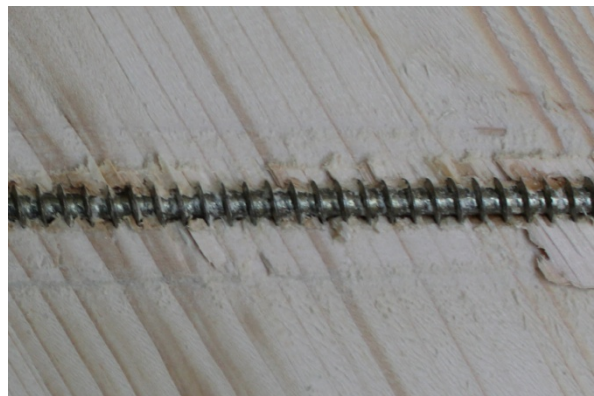
b) Probe P-20-8-6-3 d_s = 8 \text{ mm} , \alpha = 60^\circ , l_p = 200 \text{ mm}
