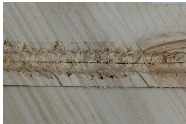
d) Probe P-18-12-6-1 d_s = 12 \text{ mm} , \alpha = 60^\circ , l_p = 180 \text{ mm}
