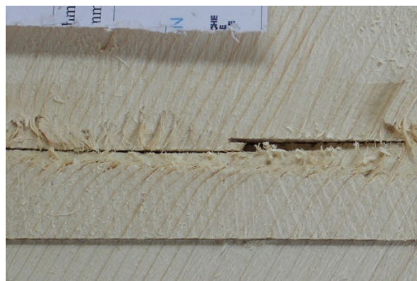
d) Probe P-12-8-6-1 d_s = 8 \text{ mm} , \alpha = 60^\circ , l_p = 120 \text{ mm}
