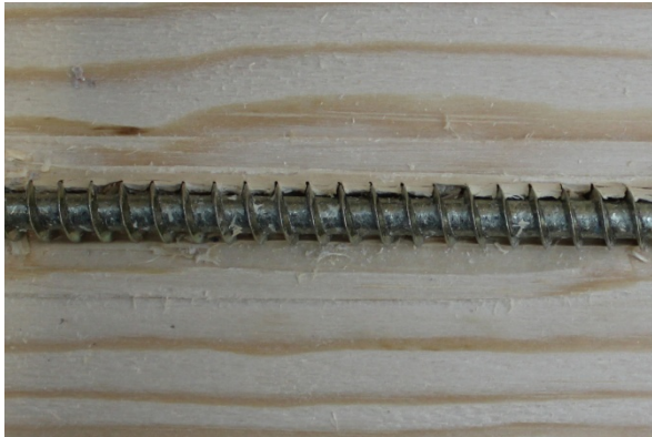
a) Probe P-25-10-0-1 d_s = 10 \text{ mm} , \alpha = 0^\circ , l_p = 250 \text{ mm}
