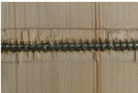
e) Probe P-25-10-9-3 d_s = 10 \text{ mm} , \alpha = 90^\circ , l_p = 250 \text{ mm}
