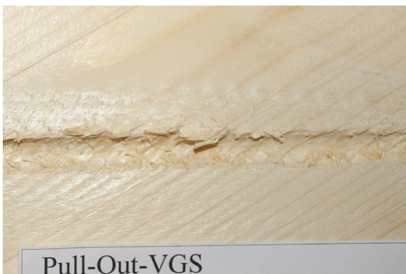
e) Probe P-16-8-3-2 d_s = 8 \text{ mm} , \alpha = 30^\circ , l_p = 160 \text{ mm}
