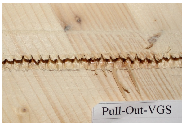
c) Probe P-20-10-6-1 d_s = 10 \text{ mm} , \alpha = 60^\circ , l_p = 200 \text{ mm}
