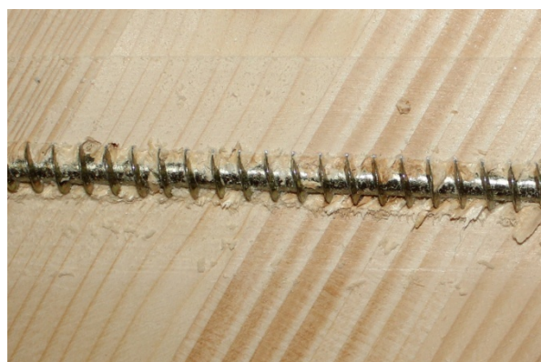
f) Probe P-25-10-6-2 d_s = 10 \text{ mm} , \alpha = 60^\circ , l_p = 250 \text{ mm}
