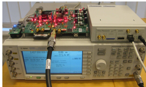
Figure D.4: The setup used to profile sensing devices with the signal fed directly over the coaxial cable. We considered different power levels and the whole range of operating frequencies. We used five devices of each type to study the variations in displayed performance between the devices.
