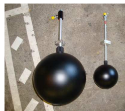
10- \ell -Kammer: \varnothing 27,0 cm 1- \ell -Kammer: \varnothing 14,0 cm
