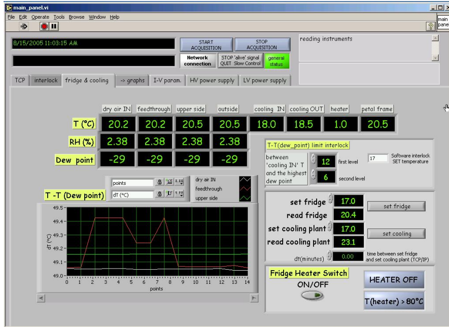
Figure 4.5: Screen shot of the slow control software. On this tab the monitoring of the temperature is shown [43].
