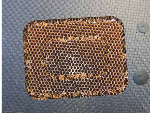
Figure 2.9: Structure of a part of petal body could be seen (NOMEX within CFC). The honey comb structure was partially destroyed during removal of the CFC skin.
