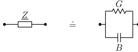
Figure B.6: Interpretation of measured impedance ( \underline{Z} ). In the context of CV measurements \underline{Z} is interpreted as a parallel circuit of conductance G and capacitive susceptance B .
