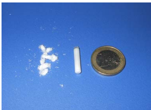
Fig. 5.2 Preparation of the Dyneema® samples used for the ^{13}\text{C} - ^1\text{H} WISE experiments.
