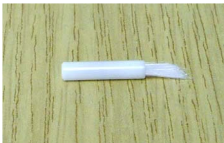
Fig. 5.1 The fibers were partially aligned along the rotor axis; the 4 mm diameter rotor is oriented inside the spectrometer's NMR probehead along the magic angle \theta = 54.7^\circ with respect to the B_0 magnetic field.
