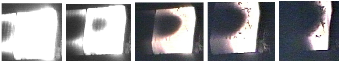
Figure 5.2 - 9. FT 107-3: Cooling down of the tile 1 after switching off the electron beam at 19 \text{ MW/m}^2
