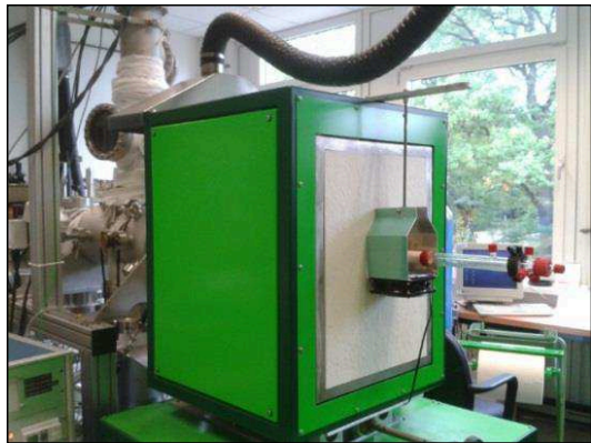
Figure 14. Atmospheric flow channel reactor coupled to an MBMS.
