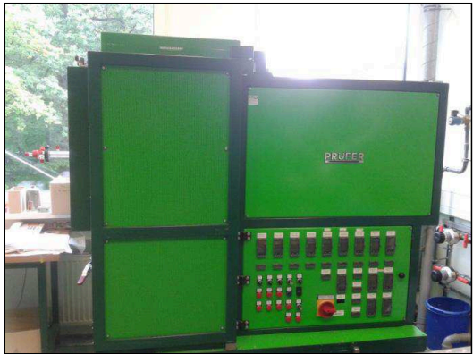
Figure 10. Atmospheric flow channel reactor with a cooling zone.
