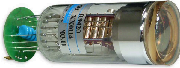
Figure 31: Photomultiplier tube for scintillation counting applications (420 nm peak sensitivity), such as PET (Hamamatsu, Japan). Diameter: 38mm. Anode to cathode supply voltage: 1500 V.
