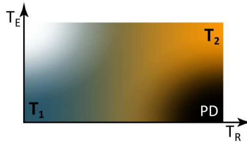
Figure 21: Graphical representation of the TE/TR - influences on the MRI image contrasts (qualitative color coding: blue: T_1 -weighted, orange: T_2 -weighted, black: PD-weighted).
