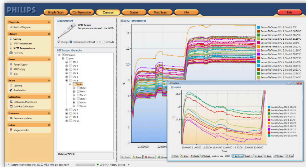
Figure 151: Control-page of the control software displaying the (d)SiPM temperatures for all 60 sensor tiles of the complete PET system. The graphs can be detached and continue in separate windows, as shown with the temperature-graphs of the humidity sensors the SPUs.
