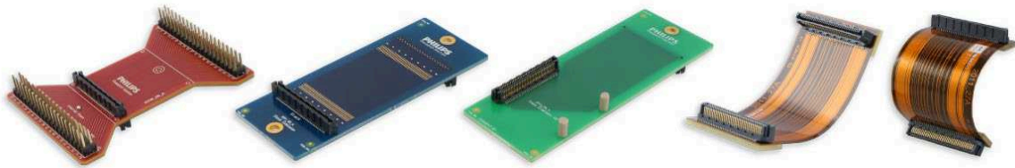
Figure 119: Different adaptors to connect a detector stack to the SPU: A debugging adaptor (left, red) routing all pins to headers, two adaptors displacing the stack horizontally (blue and green), and a flexible PCB allowing the stack to be tilted and turned in multiple dimensions.
