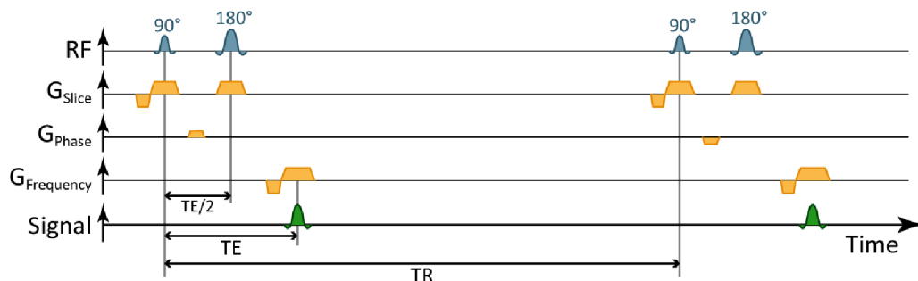
Figure 14: Simplified sequence diagram of a SE sequence
