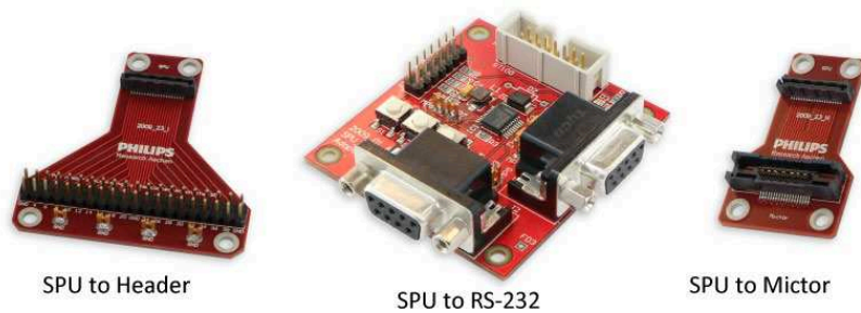
Figure 73: Debugging PCBs to connect the oscilloscopes and logic analyzer (header pins and Matched Impedance ConnectOR (Mictor)) to a small, non-magnetic, connector on the SPU. A third PCB (center) contains an RS-232 interface.
