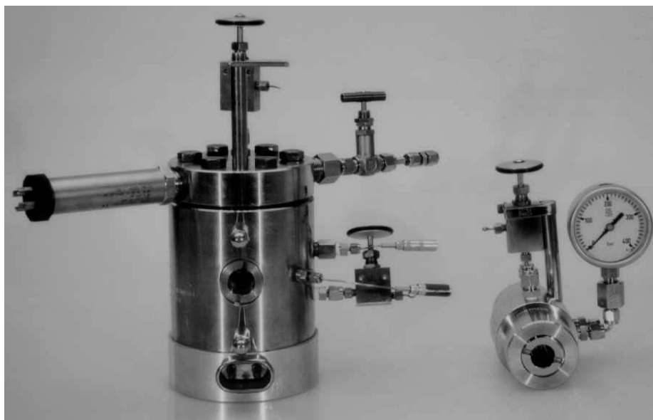
Figure 2-5: High pressure reactors used for exploratory studies on chemical synthesis using \text{scCO}_2 .
