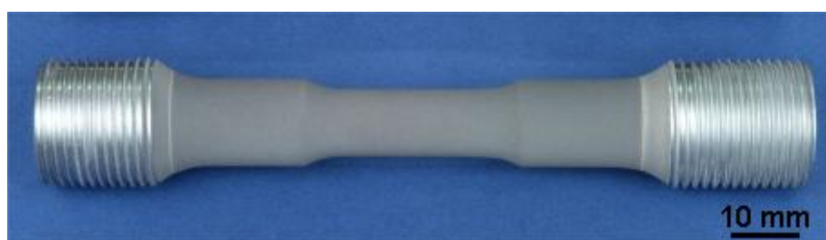
Figure 3.3 - TMF specimen configuration
