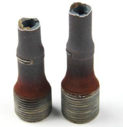
Figure 5.43 – Failure mode of TBC specimen pre-oxidized for 300 hours after OP TMF with mechanical strain range of 0.6% and temperature range of 350-1050°C
