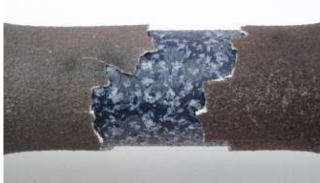
Figure 5.49 - Spallation of TBC after OP TMF with dwell time at high temperature in temperature range of 350-1050°C and mechanical strain range of 0.6 %
