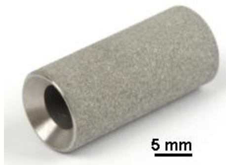
Figure 3.6 - Specimen configuration for thermal cycling
