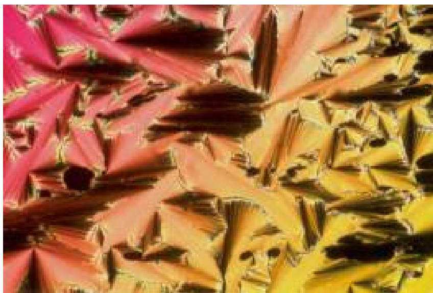
Figure 2.12 Polarized micrograph of a fan-shaped texture of a smectic mesophase.
