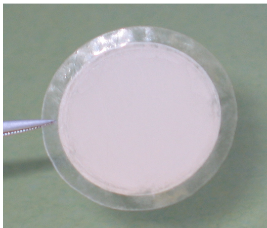
Figure 5.22 Cross-linked 16 / HMT10 (15/85wt%) on Anodisc membrane filters.
