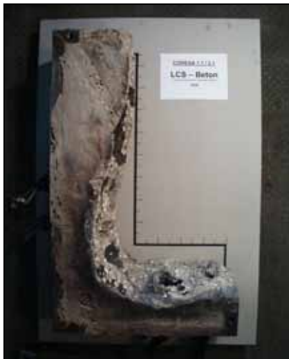
Abb. 7.2 erodiertes L-Profil, Lime-stone-Common Sand (LCS)
