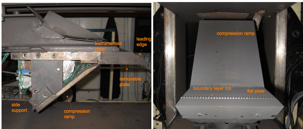
Figure 7.5. Photographs of the investigated model inside the test section of the T4 shock tunnel. Side view (left). Front view (right), this picture is rotated of 180 degrees for clarity.
