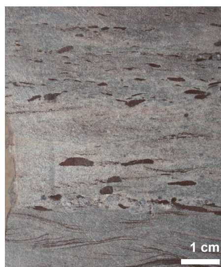
Figs. 3.16. Low energetic fluvial deposits with \epsilon -cross-stratification and clay rip-up clasts (right). N C GER, Well I.
