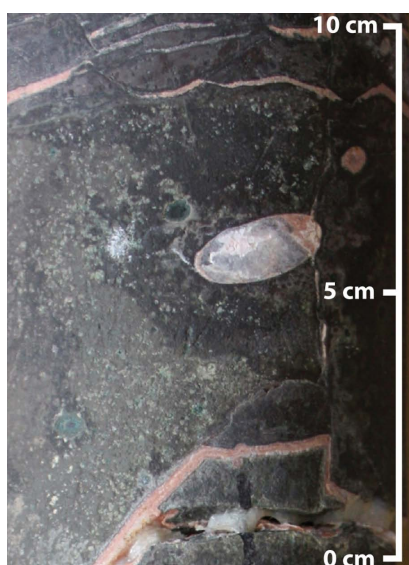
Fig. 4.7. Andesitic volcanics in core material of Well 3, underlying the reservoir succession.
