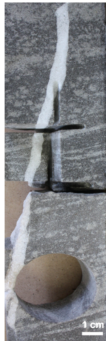
Fig. 7.6. Diagenetically overprinted dune deposit, picture from Well II.
