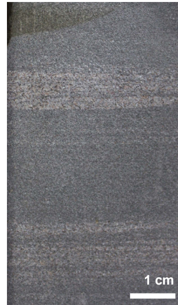
Fig. 3.11. Dry sandflat deposits with coarse grained grain flows. N C GER, Well II.
