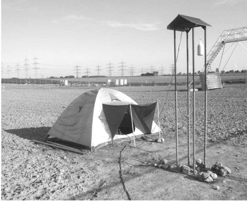
Figure 6.2: Set up for the on-field measurement of saturation. The tent contains the measurement electronics.
