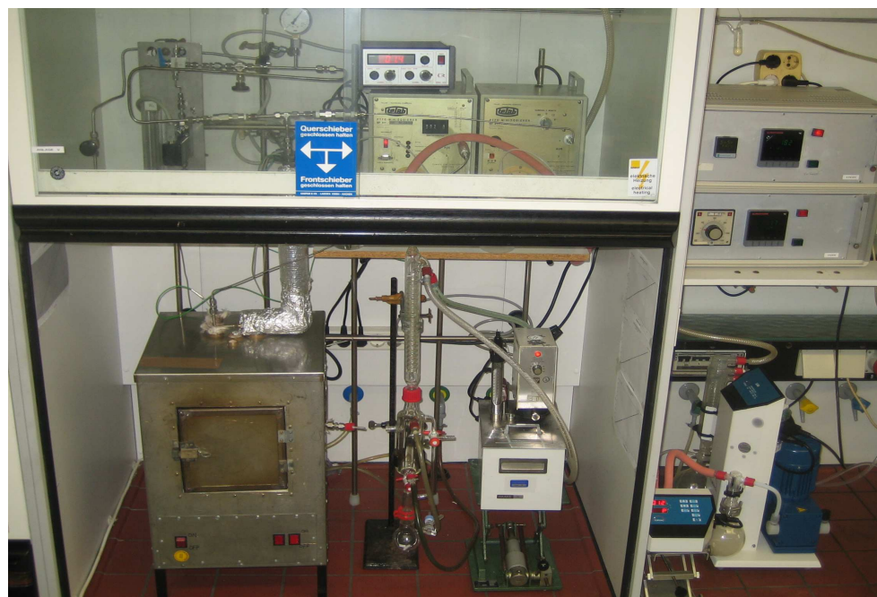
Fig. 5-2: Set-up V - liquid feed gas phase continuous flow reactor with reduced pressure.
