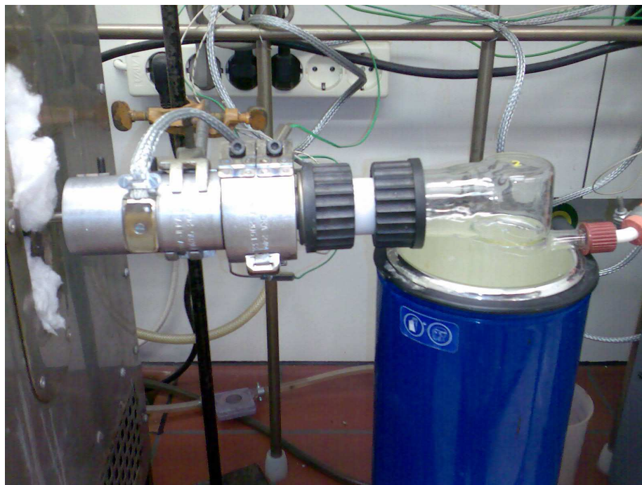
Fig. 5-4: Reactor outlet Set-up VI - liquid feed gas phase continuous flow reactor with reduced pressure
