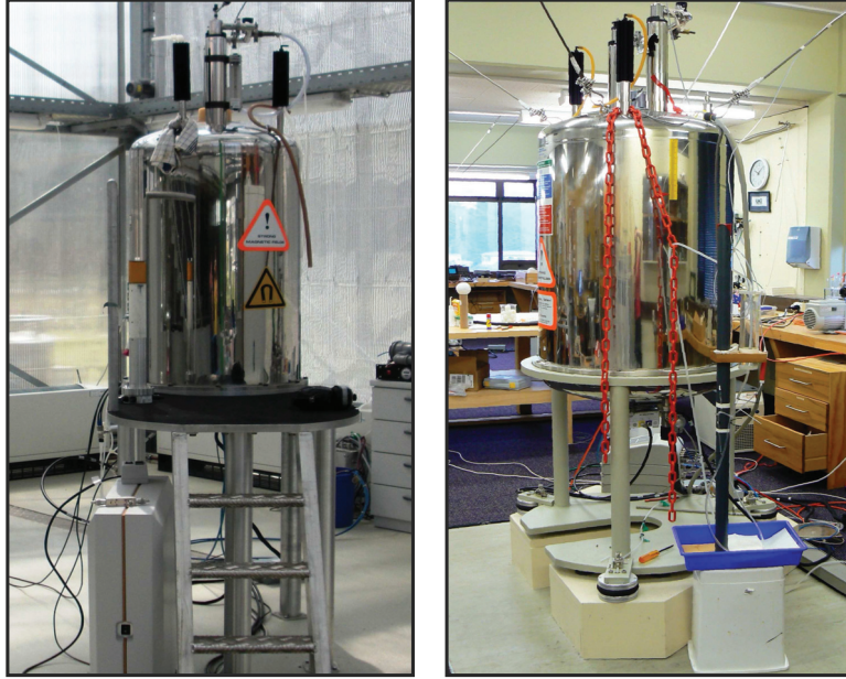
Figure 2.1: Magnet systems used for the measurements presented in this thesis. The picture of the left hand side shows the 7 T system at the Forschungszentrum Jülich, Germany. On the right hand side is presented a picture of the 9.4 T system at the Victoria University of Wellington, New Zealand.
