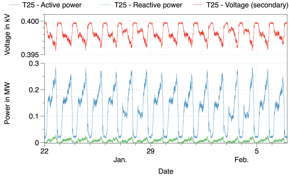
Figure 4.25: Active and reactive power flow as well as secondary voltage at a transformer (T25) of the model of the city district energy system for a time period of 16 days for the reference scenario
