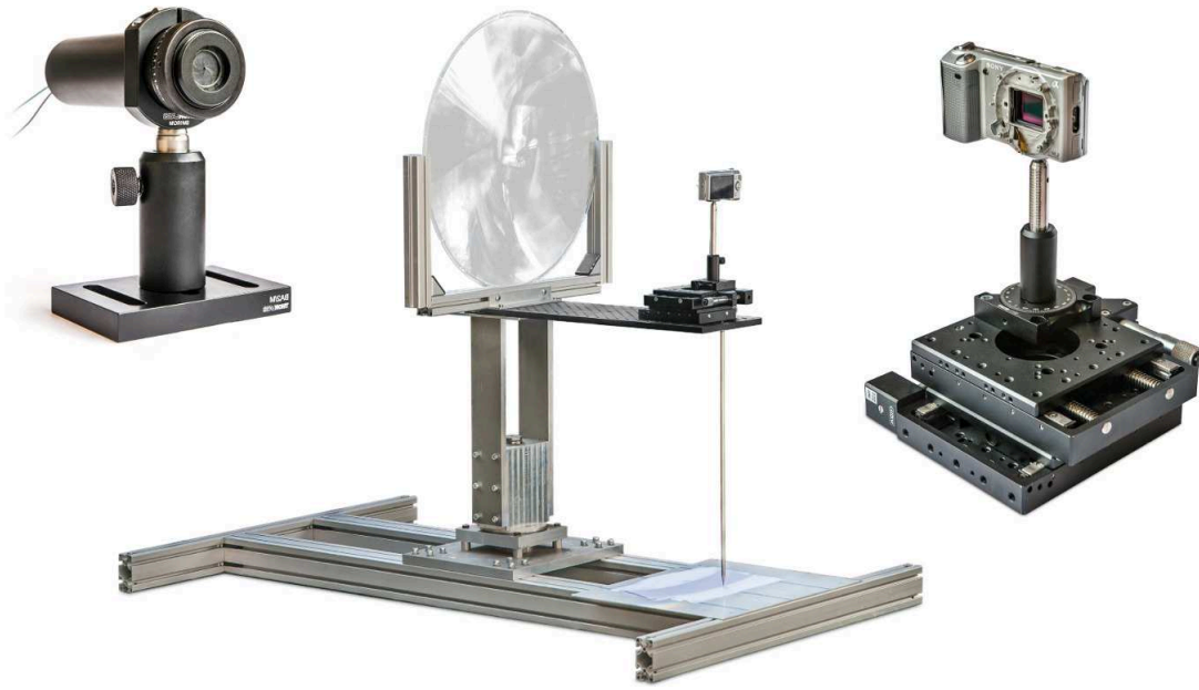
Figure 6.4: Photographs of the main parts of the setup for the measurement of the PSF of the Fresnel lens. Adapted from [150]. Left: the green LED used for the measurements is placed inside a light-tight tube behind a pinhole adjustable iris. Middle: the Fresnel lens is fixed in a frame and mounted onto a rotary table. The camera is situated behind the lens on its optical axis on the same rotary table. Right: the position of the camera can be finely tuned by means of translational stages.
