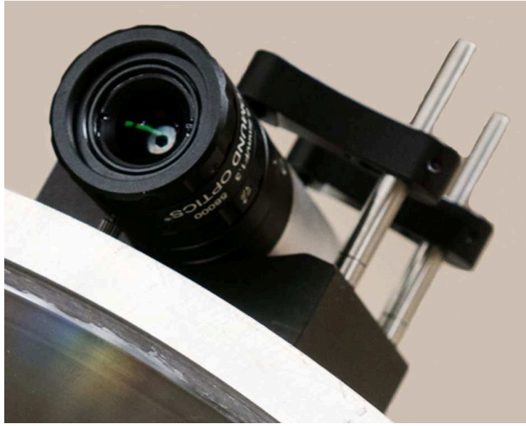
Figure 6.19: Photograph of the night sky camera of FAMOUS mounted on the telescope tube. Attached to the QHY5L-II-C CMOS camera is a fixed-focal-length lens from Edmund Optics. The sensor is read out continuously via USB and the photographs of the night sky are stored for further analysis of the visible stars in the field of view. The field of view is roughly two-fold of the field of view of FAMOUS.
