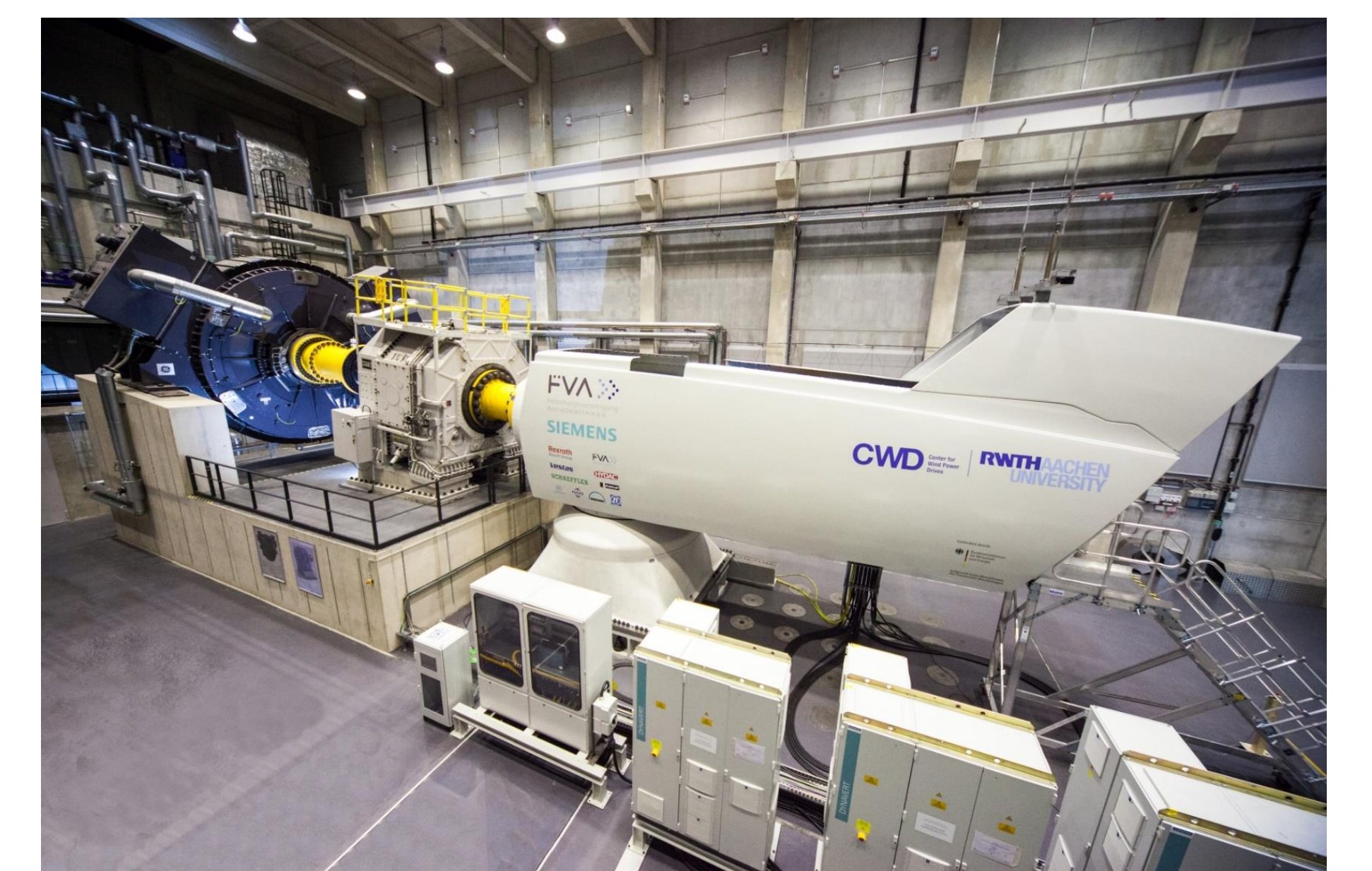
Device under test on the 4MW WTG system test bench
