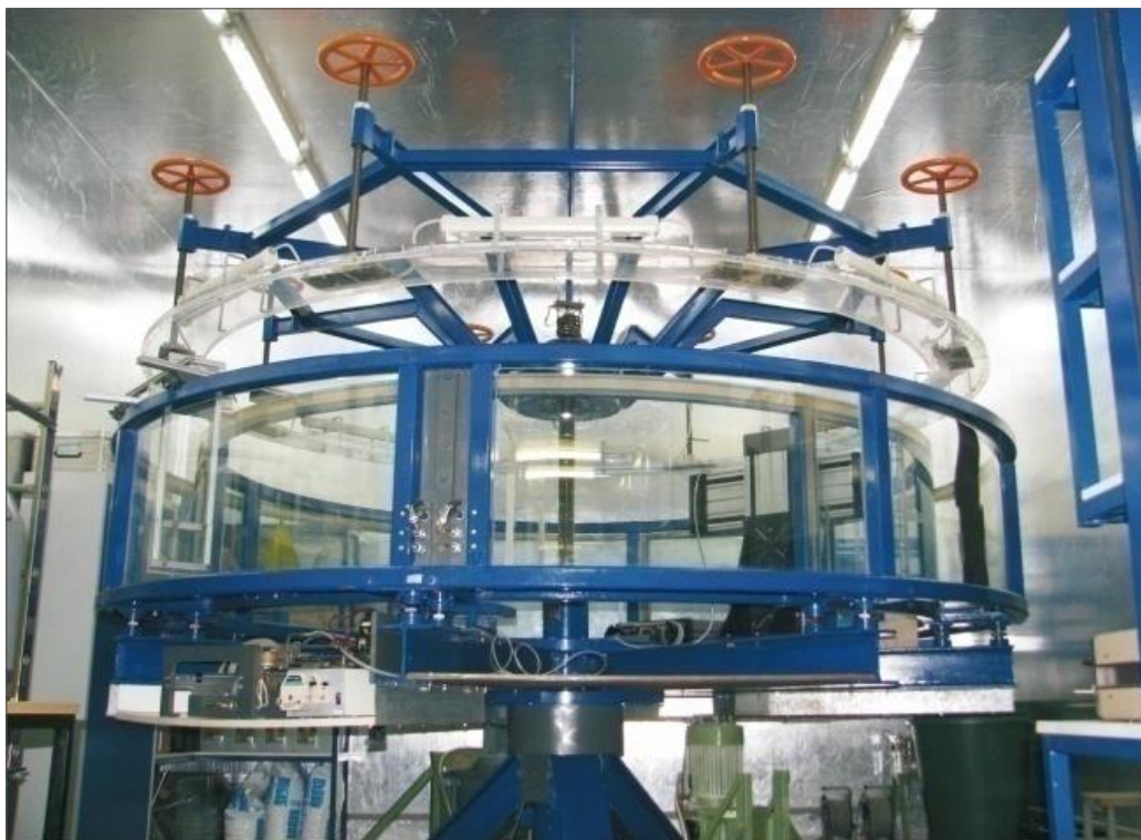
Figure 3.1: Annular flume at the Institute for Hydraulic Engineering and Water Resources Management, Aachen, Germany; Picture: C. Cofalla.
